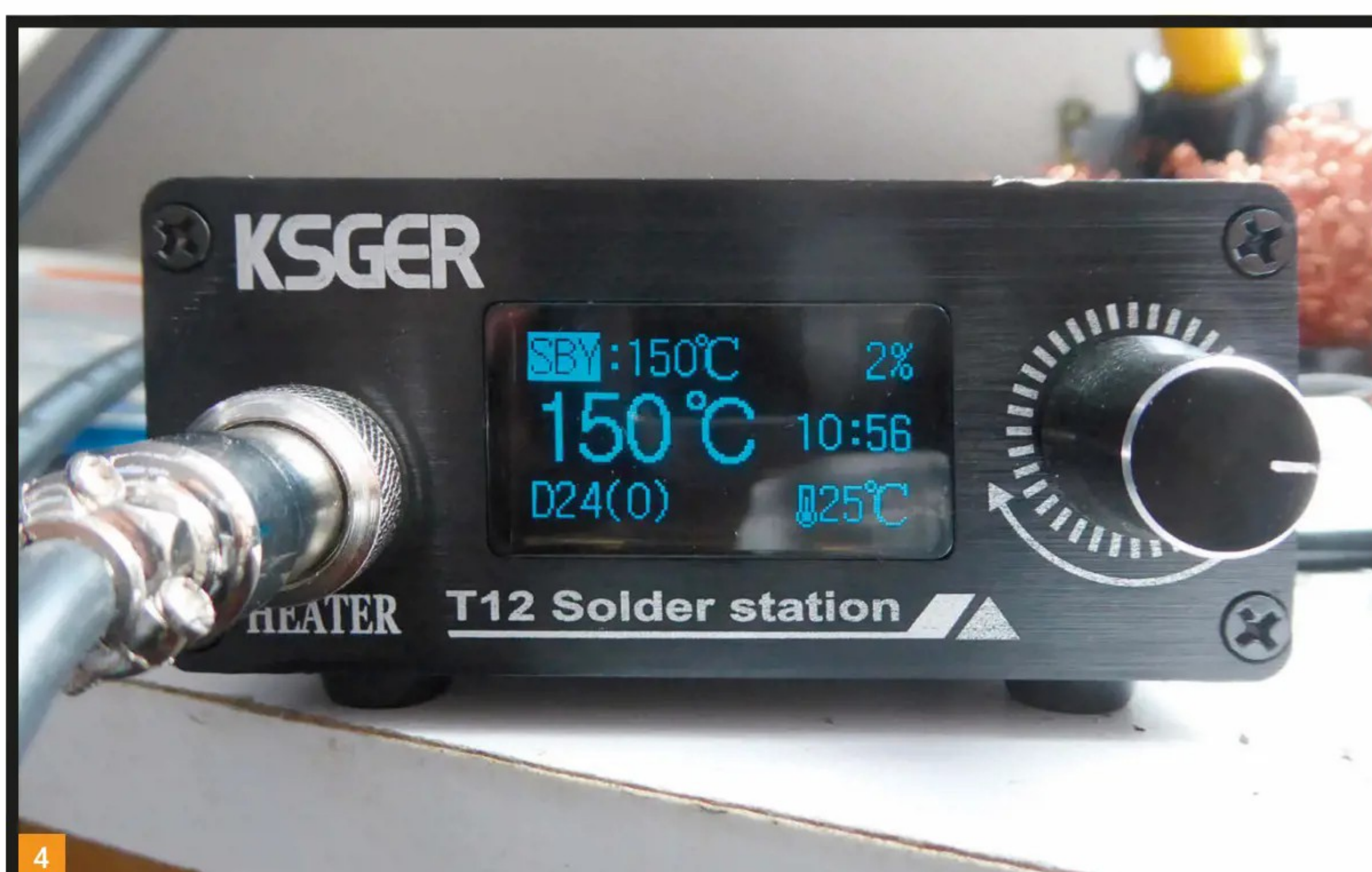
Fig. 1: The KSGER as supplied. Fig. 2: The popular Weller soldering station. Fig. 3: In the hand. Fig. 4: Front Panel showing Standby, Target Temperature of 150°C, Actual Temperature, Percentage power being applied, Fitted tip (D24), CPU Temperature and the time. Fig. 5: Internal view.
