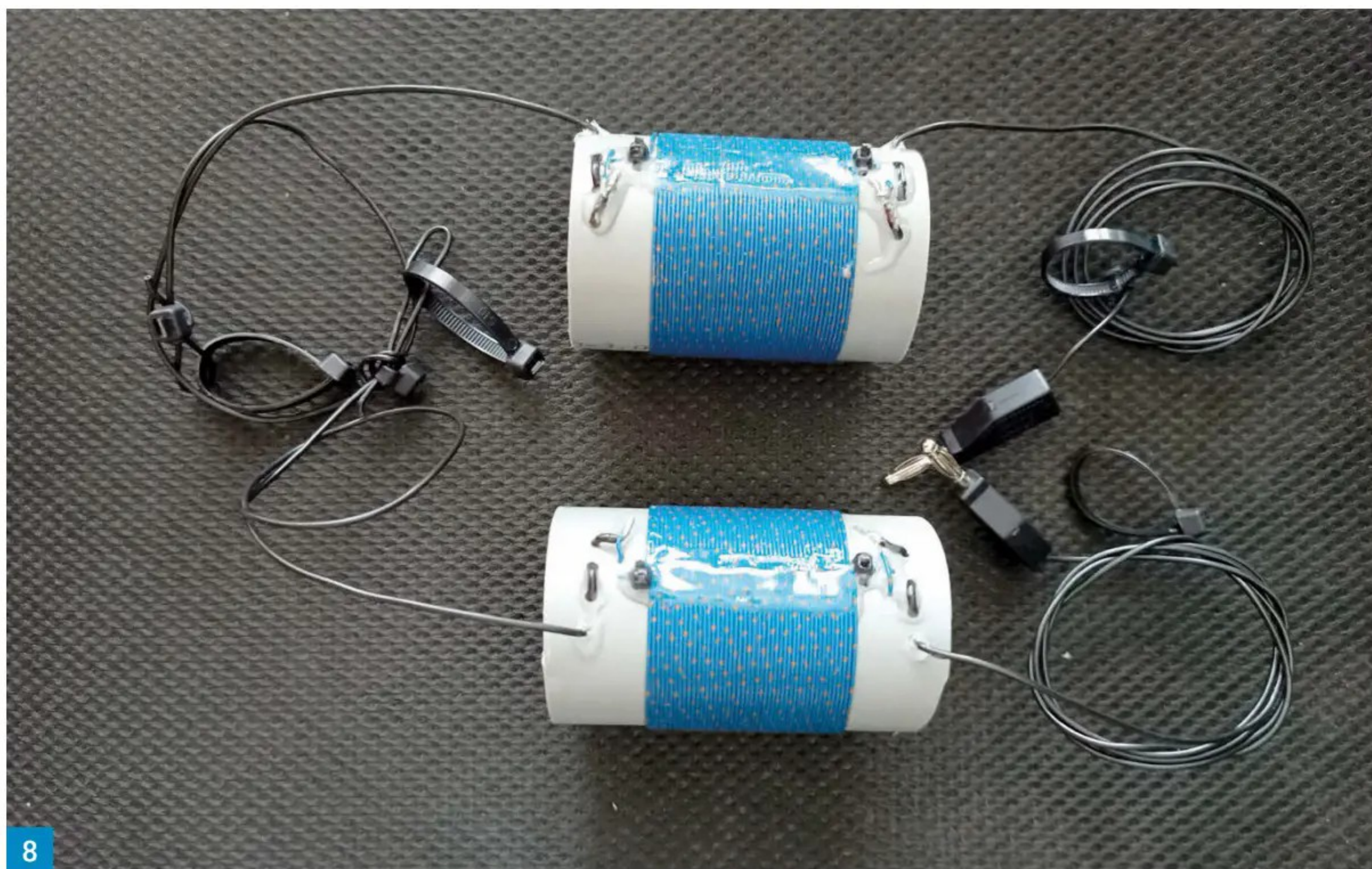
Fig. 8. Finished 40m loading coil, one needed for each leg of the dipole.
