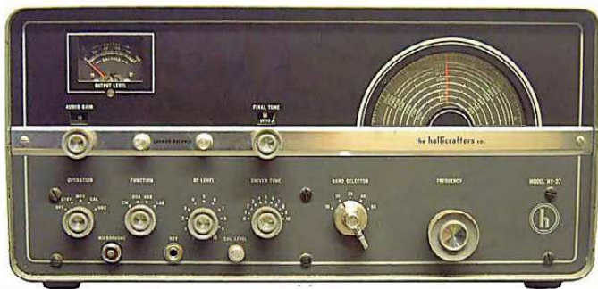
The HT-37 used the phasing method of sideband generation, while the HT-32 family used a crystal-lattice filter to generate SSB. [Photo courtesy of www.rigpix.com ]
