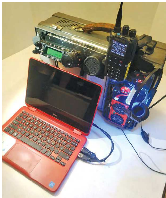
This all-band go-kit includes a radio, antenna tuner, laptop, battery management system, accessories, safety features, and more.
