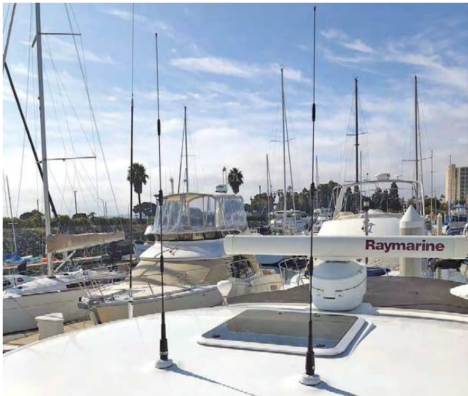
The hamstick-style antennas for VHF and UHF, custom mounted on the roof of the boat.
